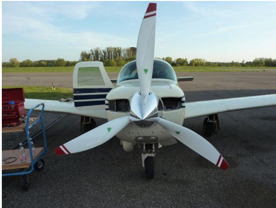
Propeller B: : MT - MTV-12-D Propeller with internal De Ice system (Villinger)
