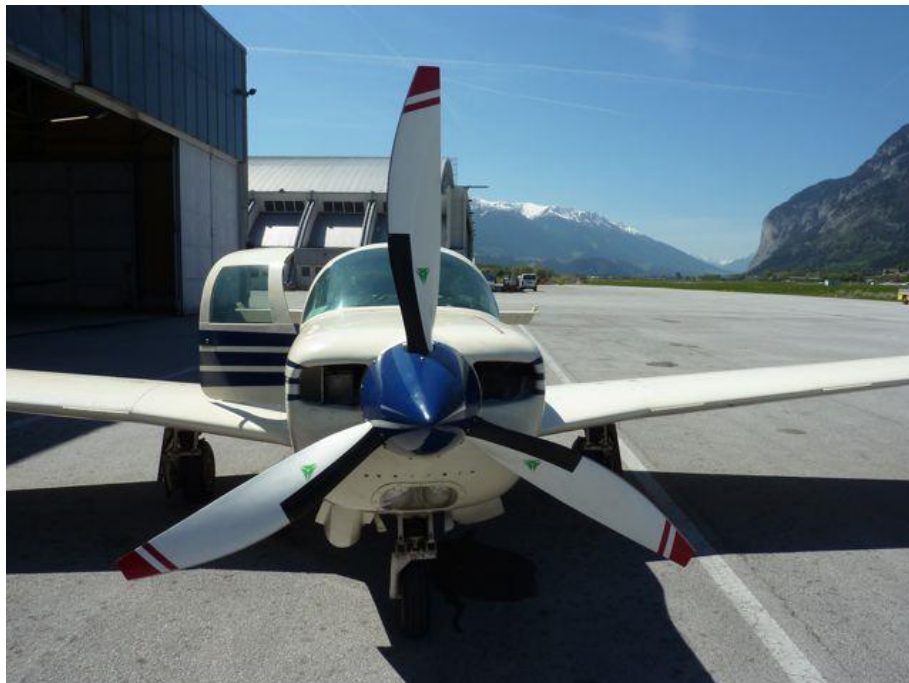
Propeller A : MT - MTV-12-D Propeller with conventional De-Ice boots (Goodrich)
